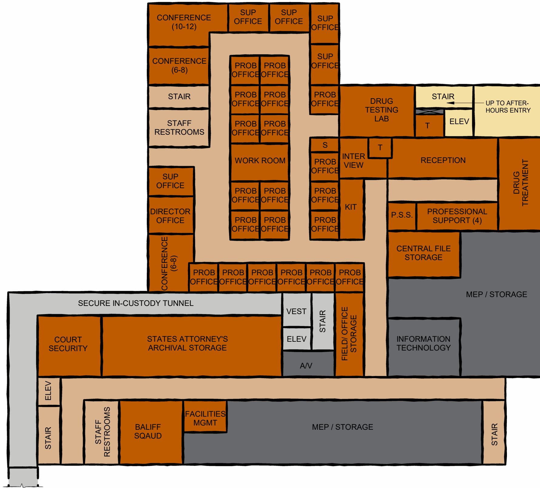
1 NEW JUSTICE CENTER ANNEX - OPTION F-3 - BASEMENT LEVEL FLOOR PLAN 1" = 20'-0"
